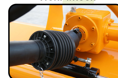
▶ Freewheel on transmission
